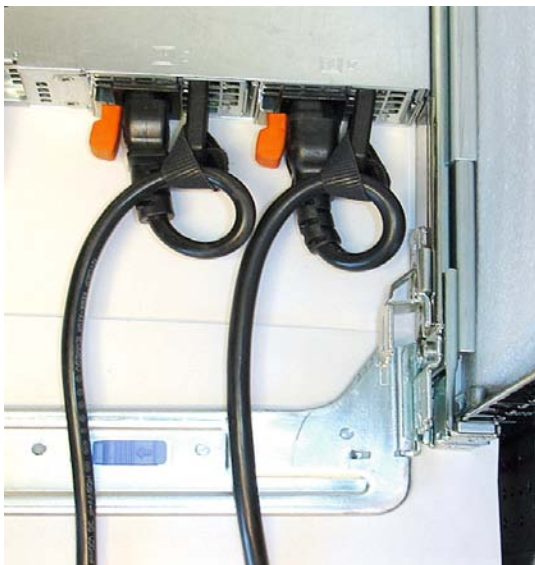
Figure 3: Routing Power Cables Through the Strain Reliefs
